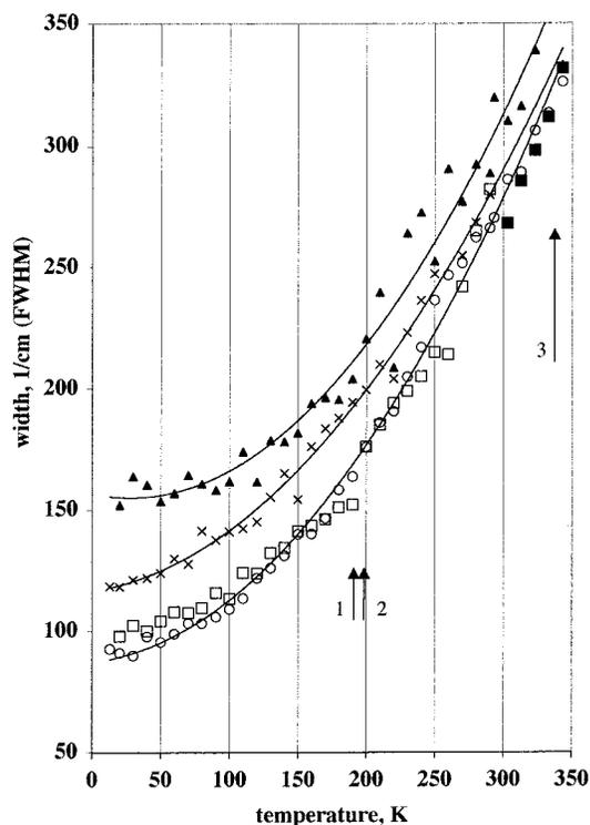
**Figure 7.** Absorption widths of the Q(0,0)<sub>x</sub> band of Fe(II) cyt *c*. The protein was in the following matrix: closed squares: water; open circles: 60% glycerol/water (glass transition indicated by arrow 1); open squares: trehalose formed at 193 K (glass formation temperature indicated by arrow 2); x: trehalose formed at 333 K (glass formation temperature indicated by arrow 3); closed triangles: trehalose formed at 373 K. Lines are polynomial fits and serve only as a visual aid.
