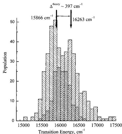
**Figure 12.** Effect on the optical transition including distortions of the heme and the fluctuation electric field due to charges of the protein, Fe-porphyrin-Q. Populations of calculated transition energies were calculated for the structures from the dynamics simulation. Lower transition and upper transition are distinguished by angle of the shading.
